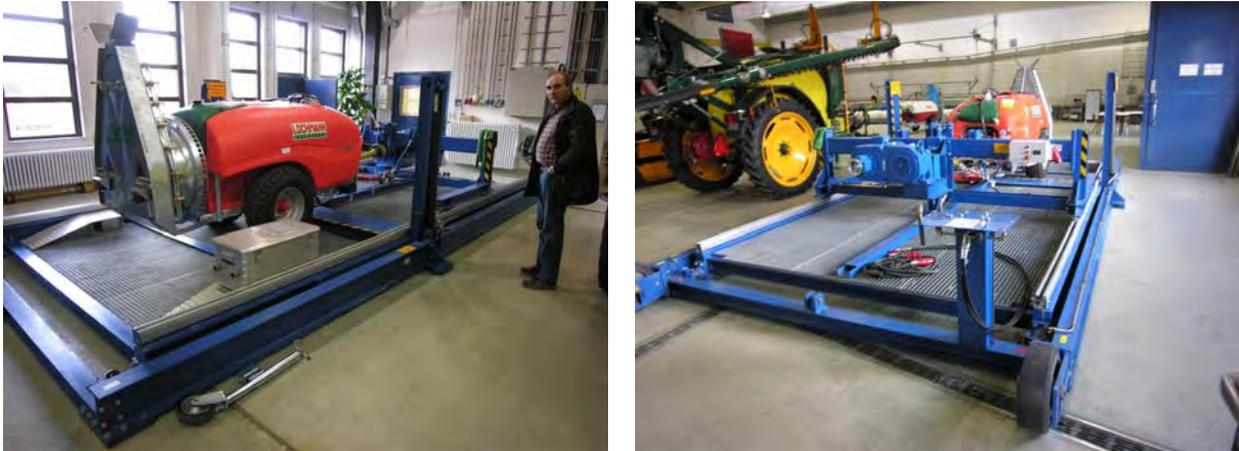
Photo 2. Tilting floor for spray residual measurement.
