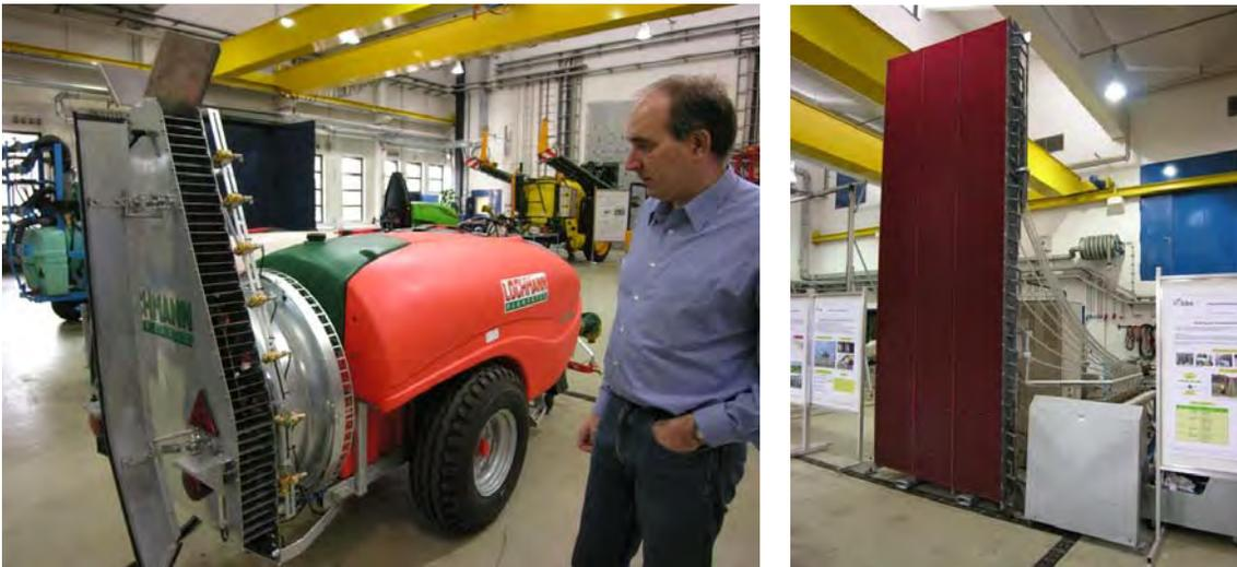
Photo 1. Dirk Rautmann with shielded orchard sprayer and vertical collection system (patternator).
