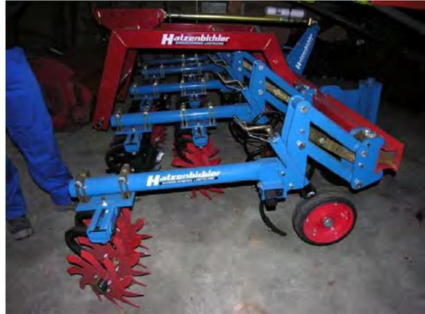
Photo 4. Hermann Scheb-Wetzel and Hatzenbichler front mounted inter-row cultivator
