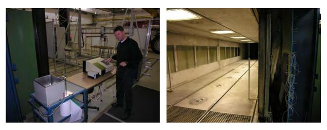
Photo 3. Andreas Herbst measuring drift using an ultra-sonic bath (left) and wind tunnel (right)
