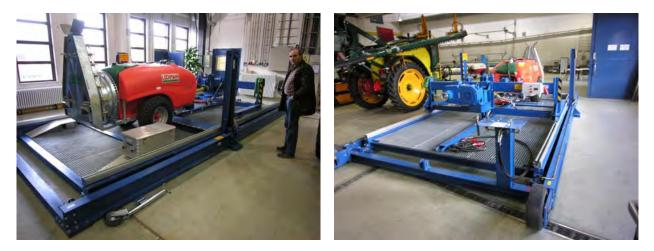
Photo 2. Tilting floor for spray residual measurement.
