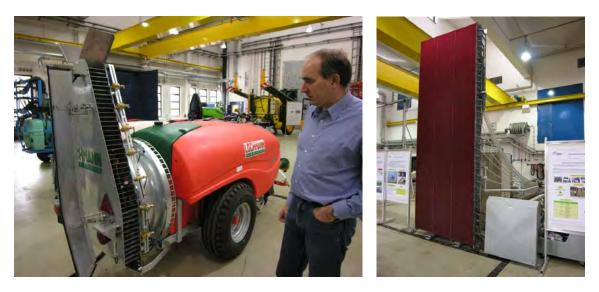
Photo 1. Dirk Rautmann with shielded orchard sprayer and vertical collection system (patternator).
