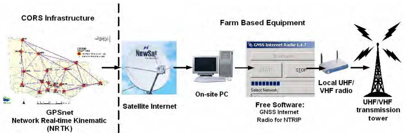
Figure 4. Modular system components of the re-broadcast model
