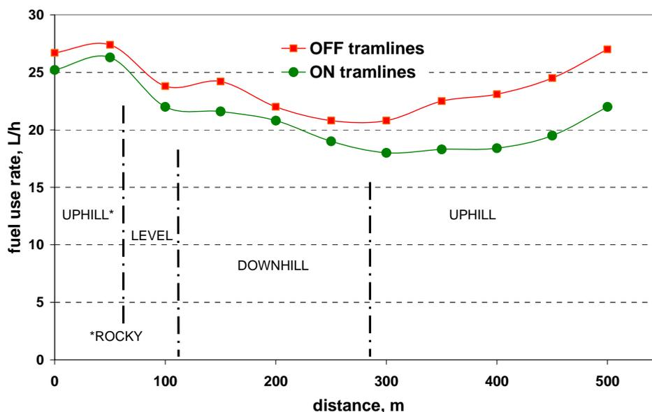
Figure 1. An example of fuel use with or without tramlines for a herbicide spraying operation at Minninooka farm near Geraldton. The effect of slope on tractor movement is indicated, as well as the surface condition. Tramlines reduce fuel use by reducing rolling resistance.
