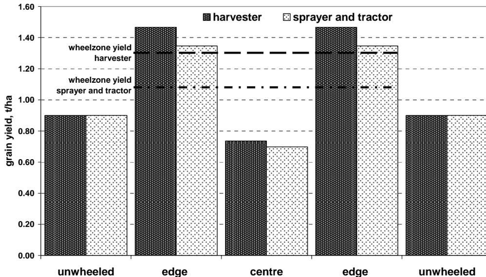
Figure 3. Effects on yield by traffic on deep ripped sand in a dry season. The harvester was used in the previous season, the sprayer before seeding. The 'wheel zone' is twice the wheel width and 'edge' measurements came from the unwheeled crop next to the wheelmark and half the width of the wheelmark. 'Centre' is the central 50% of the wheelmark
