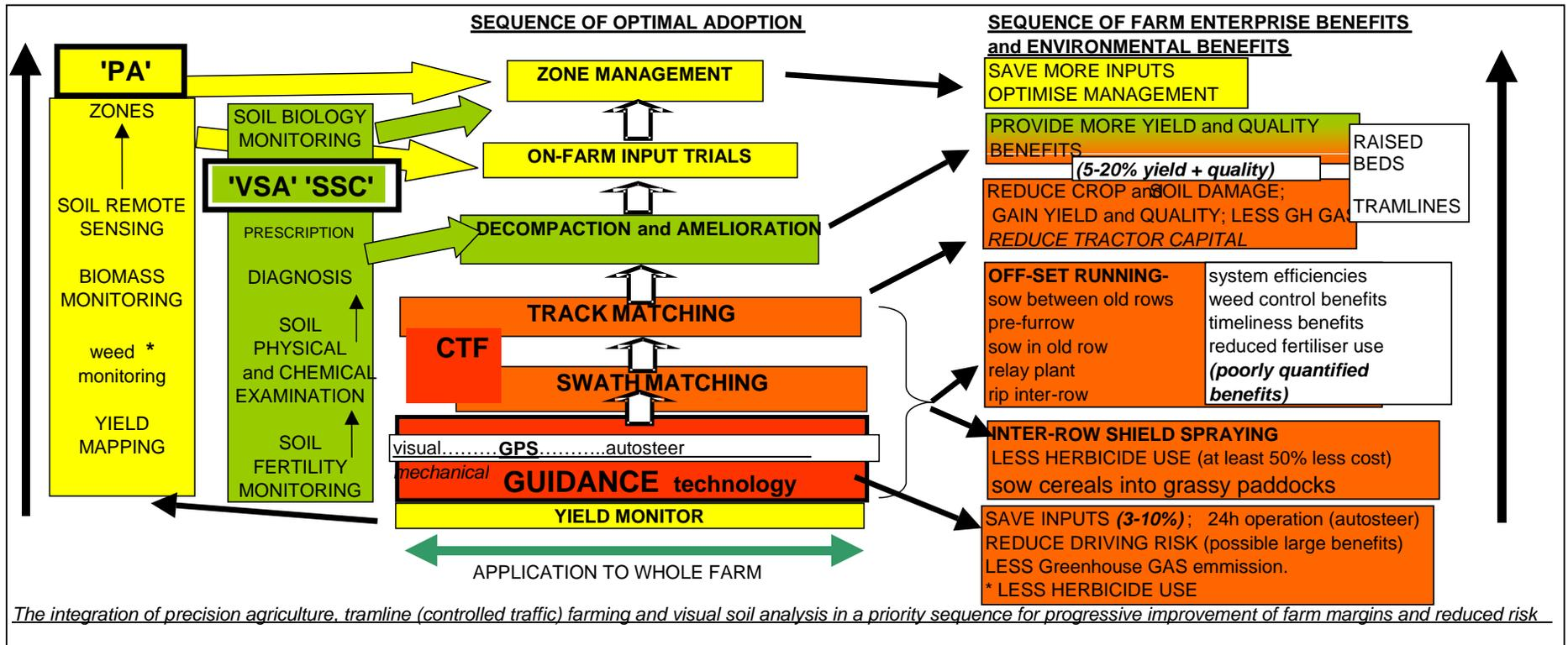
Figure 5. A flowchart showing the integration of Controlled Traffic Farming, Precision Agriculture and subsoil improvement
