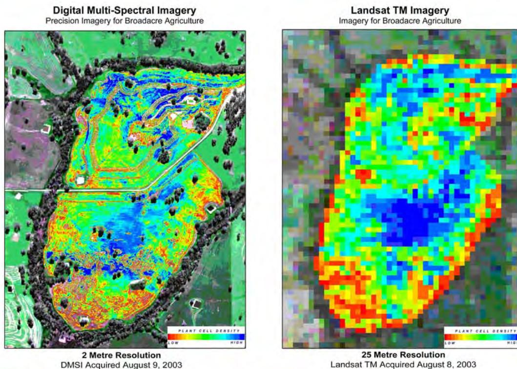
Figure 1: The advantage of high resolution Digital Multi-Spectral Imagery (DMSI) over satellite systems
