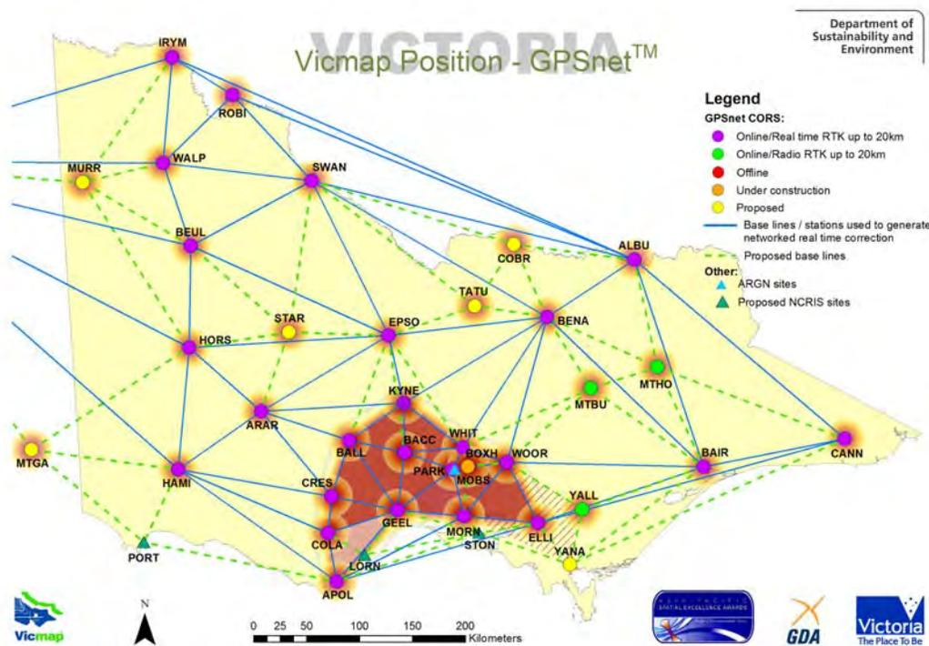
Figure 1. Victoria's CORS network, GPSnet
