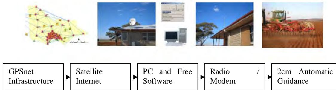
Figure 2. CORS NRTK system for 2cm automatic guidance
