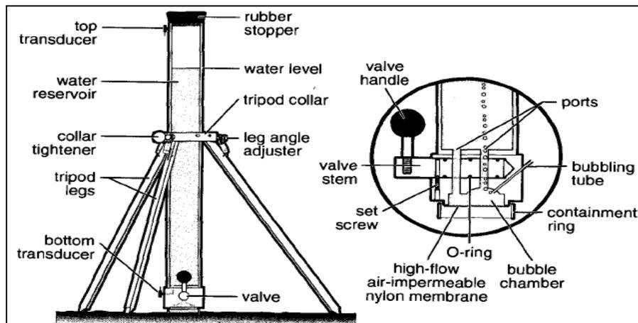
Figure 1. Schematic diagram of the single-ring infiltrometer (*image courtesy of Fangmeier, et al.*)
