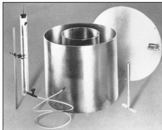
Figure 2. Double-ring infiltrometer (*image courtesy of [www.rickly.com](http://www.rickly.com)*)
