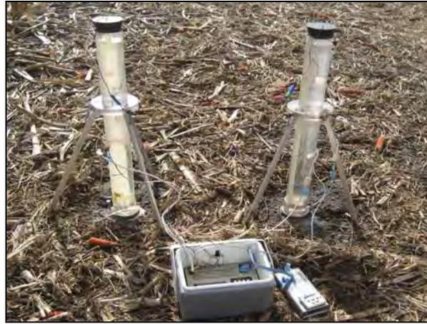
Figure 3. Water infiltration data collection
