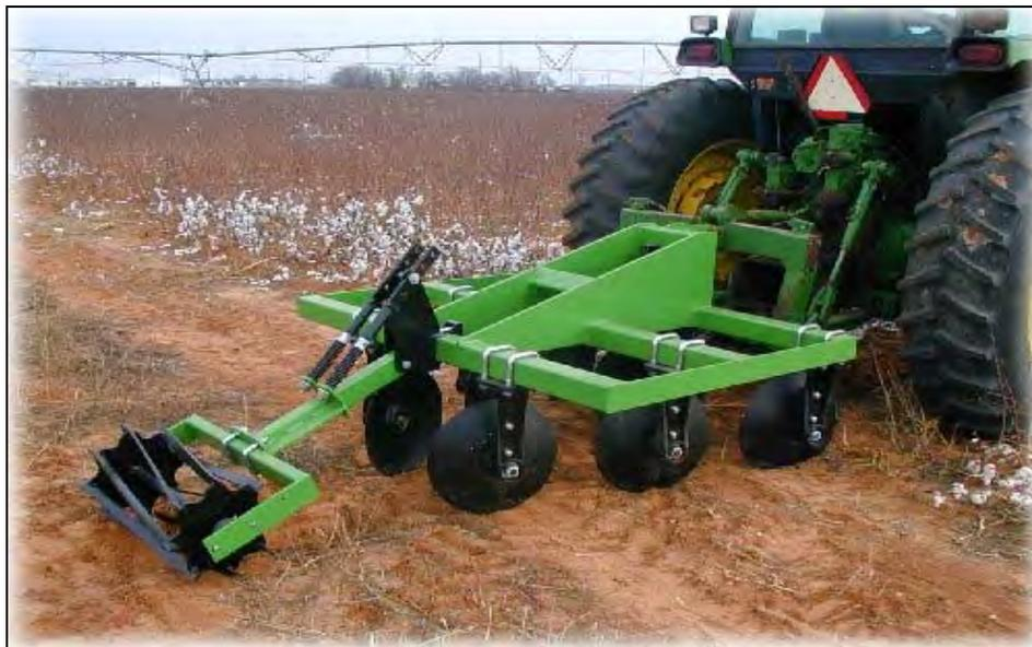
Figure 16. Bigham Brothers pivot track disc filler (image courtesy of <http://www.bighambrothers.com/trackfiller.htm>)
