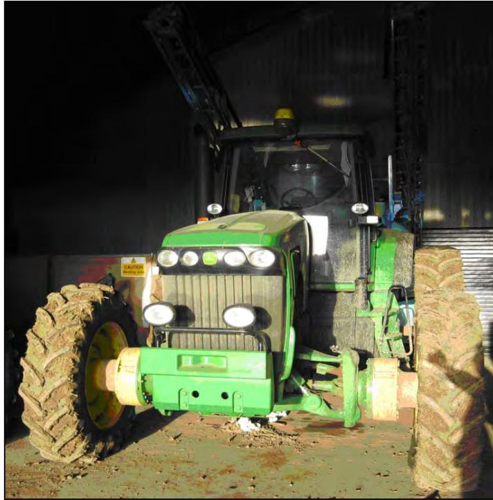
**Figure 17. Tractor configured for 3 meter (120 inch) CTF**
