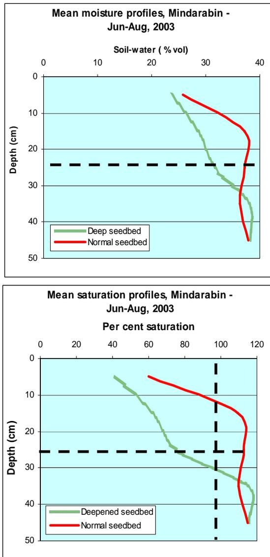
Figure 6. Average soil moisture profiles in a deepened seedbed and normal seedbed in a grey clay soil at Mindarabin WA
