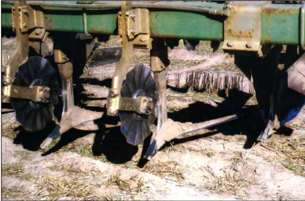
Figure 1. Ripper with narrow, widely spaced tines and wide blades that is used to maintain deepened loose seedbeds with near-ideal physical conditions in soils with shallow, dense ploughpans or B-horizons.
