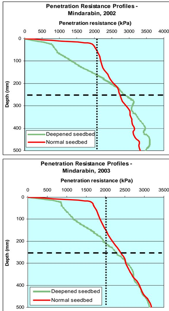
Figure 2. Average penetration resistance profiles for a grey clay at Mindarabin WA for 2002 (a very dry season) and 2003 (a wet season). The depth of the loosening is shown (horizontal dashed line), as is the penetration resistance that limits roots proliferation (2000kPa) (dashed vertical line).
