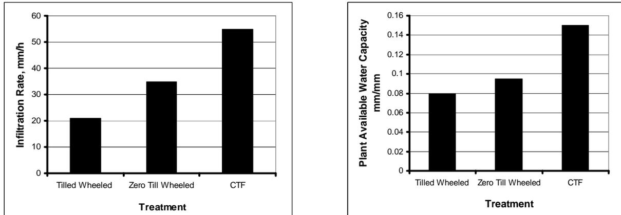
a) Infiltration rate during 80 mm/hour rainfall event      b) Plant available water capacity (0 - 30 cm after two years CTF.)
