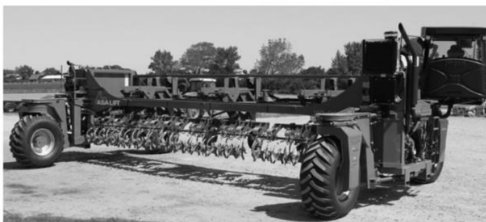
A 9.6 m Wide Span prototype tractor developed by ASA-Lift. It will be tested in all operations of onion production.
